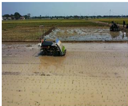
Figure 1. Rice transplanting robot (Source: BB Padi, 2019)
